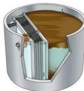
Figure 17 : Micro station à culture fixée (EPUR®)
